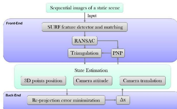
The front-end takes images as input and construct a state estimation which includes 3D point positions and camera poses. The back-end optimizes the state estimation by minimizing the reprojection error of all measurements.
