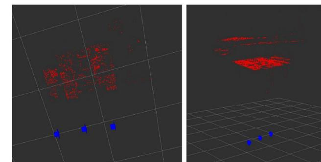
Here is our reconstruction result shown on RViz software. The three blue arrows are cameras and the red points are 3D points. The direction of the arrows show the direction of the x-axis of the camera frame. The points shows the wall at the back, the pictures hanging before the wall, and the board on the left.
