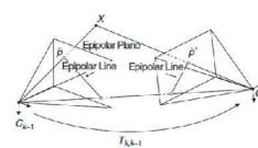
For multiple images, in order to preserve scale, *Perspective N-Points (PnP)* algorithm is implemented. With correspondence between constructed 3D points and 2D features in the new image, the pose of the new camera can be calculated without losing scale. New 3D points can then be reconstructed and successfully merged to the old points.
